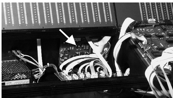
Picture 2: Please dismount the module. Now you can change R004D (40pin) to the new PIC R004D-6.3.2 in the USB interface (for the additional fader pack the new is PIC R004D-6.3.1E).
